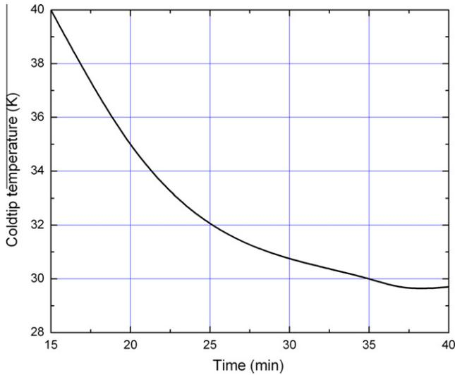
Fig. 5. Detailed cool-down process below 40 K.
