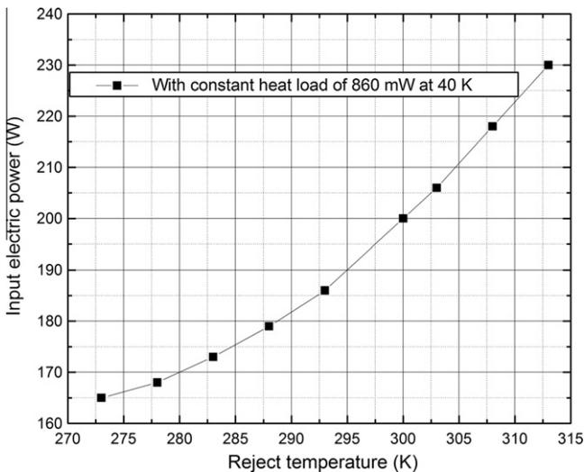
Fig. 6. Cooler's sensitivity to heat sink with constant heat load of 860 mW at 40 K.
