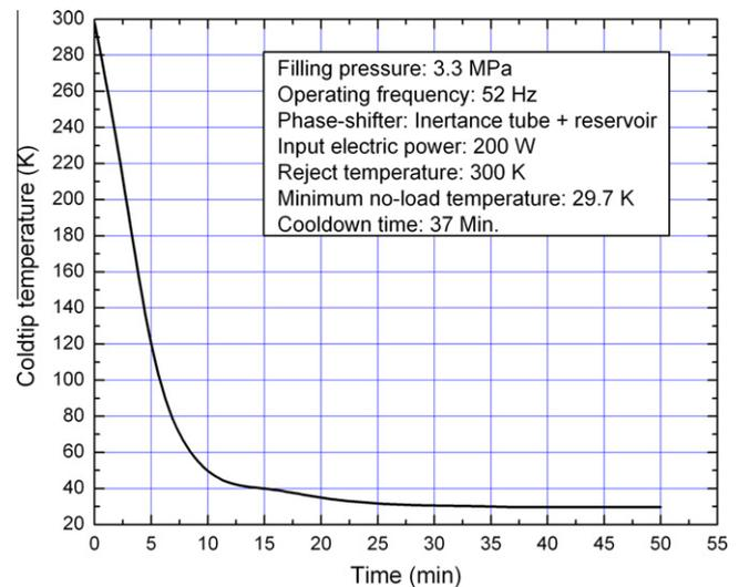
**Fig. 4.** Typical cool-down curve of the developed 40 K PTC.
