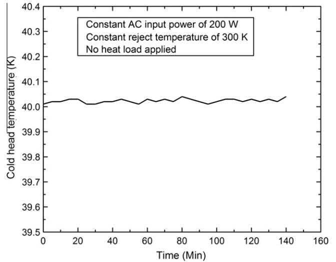
Fig. 7. Temperature stability of the developed 40 K PTC during 150 min.
