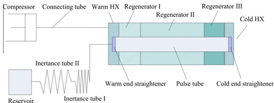
**Fig. 1.** Schematic of the developed single-stage coaxial inertance 40 K PTC.
