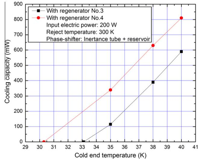
**Fig. 3.** The comparison experiments with regenerators No. 3 and No. 4.
