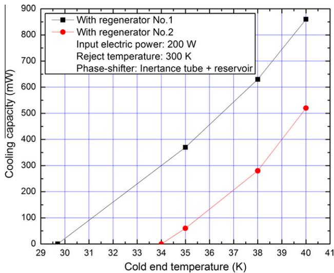
**Fig. 2.** Cooling performance of the developed PTC with regenerator No. 1 at several typical temperatures (performance with regenerator No. 2 is also shown for comparisons).
