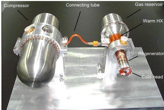
Fig. 5. The engineering model (EM) of the developed PTC.
