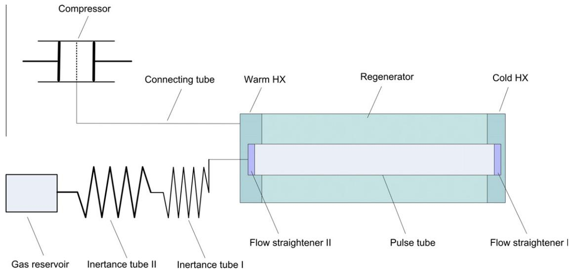
**Fig. 1.** Schematic of the high frequency PTC with three typical geometrical arrangements.
