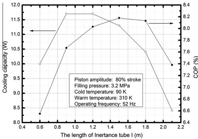
**Fig. 2.** Simulation results of variations of COP and cooling capacity at 90 K with the length of Inertance I.
