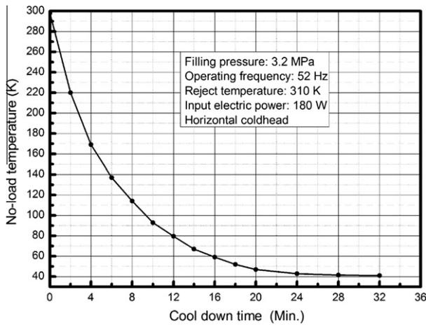
Fig. 6. The typical cool-down curve.
