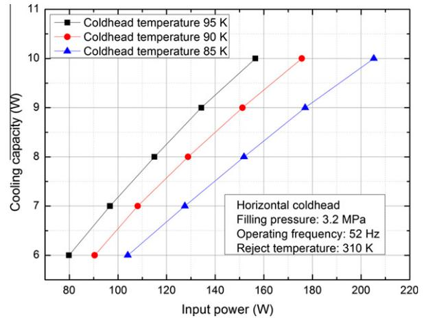
Fig. 7. Typical experimental performances at 85 K, 90 K, and 95 K, respectively. Horizontal cold head. 310 K reject temperature.
