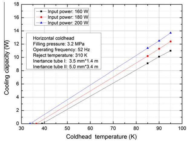
**Fig. 4.** Simulation results of cooling performance based on the optimized inertance tube dimensions.
