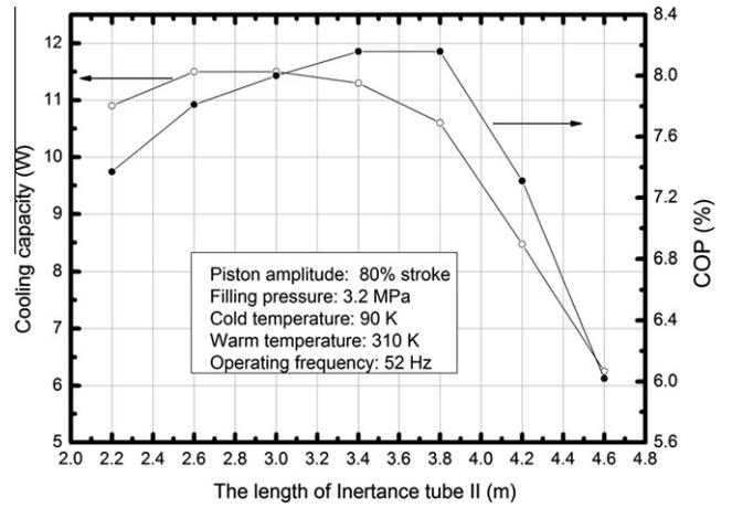
**Fig. 3.** Simulation results of variations of COP and cooling capacity at 90 K with the length of Inertance II.
