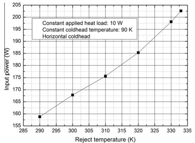
Fig. 8. Reject temperature dependence experiment with constant heat load and cold temperature of 10 W and 90 K, respectively. Horizontal cold head.
